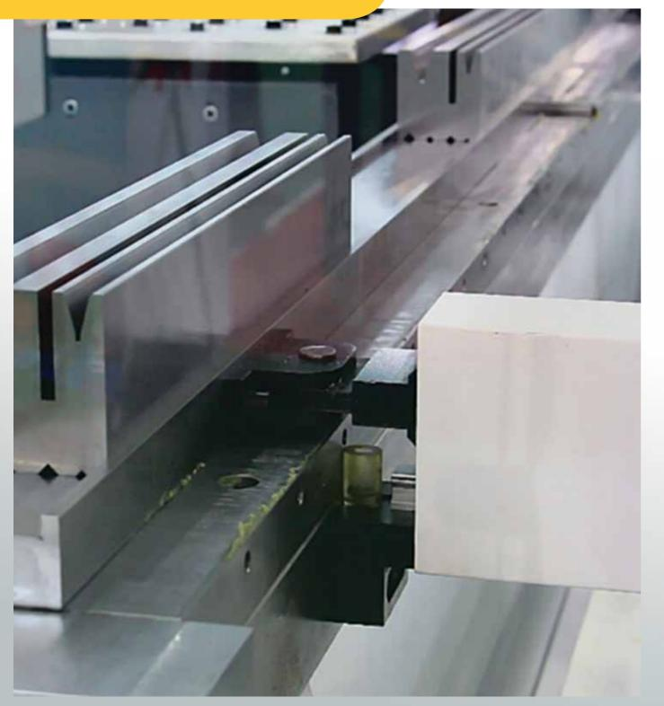
PTP2 Servo controlled table, to easy complete small bends, Using different V-openings in a die. Accurate positioning and reduced tool changes
