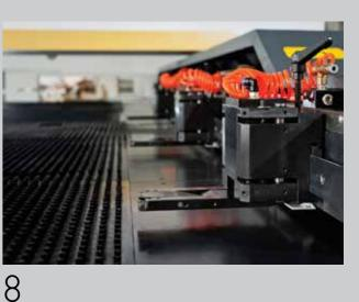
CLAMPING Movable pneumatic clamping.
