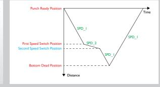
The servo-electrical punch ram allows programming of the punch operation according the exact requirements:
