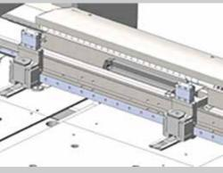
Vacuum suction of the punch scraps: Automatic clamps reposition mechanism: allows effectively suck out the punch scraps the machine to automatically position the clamps from the dies.
